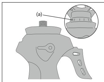
The Primos two point gun rest turns a tripod with 1/4-20 thread mounts into a full gun rest. To attach to the Primos trigger sticks unscrew the green section (a) below the V-Yoke. This will reveal the threaded section of the Trigger Stick.
