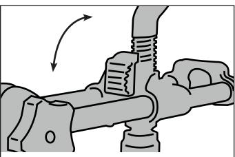
The green clips enable the V rests to be folded down for storage.
