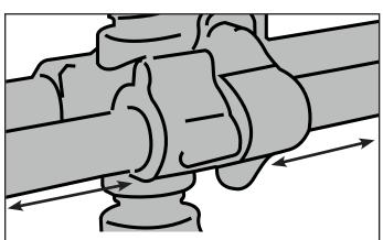
To adjust the distance between the V rests there are clips at the side of the rest which can be unclipped and adjusted.
