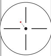
Look through the scope at the target. Adjust the scope until the laser is in the middle.
