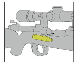
Insert the laser into the chamber and slide the bolt forward to hold the laser in place. This will activate the laser.
