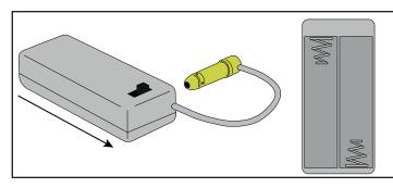
Adding the batteries to the rimfire. Slide the bottom of the sight-rite and then insert the 2 supplied AAA batteries into the sight-rite as shown.
