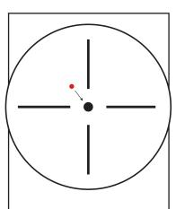
Look through the scope at the target. Adjust the scope until the laser is in the middle.
