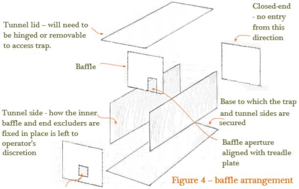
External tunnel end hole - size and position left to operator's discretion
